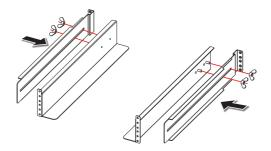
(Figure 3-2: Adjust the Rails' Length and Tighten the Nuts)
