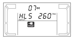
Parameter 2 & 3: Set an acceptable high voltage point and a low voltage point for bypass mode by pressing the ON/ MUTE or SELECT button.
