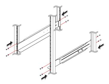
(Figure 3-3: Attach the Rails to Your Rack)
