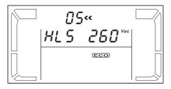
Parameter 2 & 3: Set an acceptable high voltage point and a low voltage point for ECO mode by pressing the ON/ MUTE or SELECT button.
