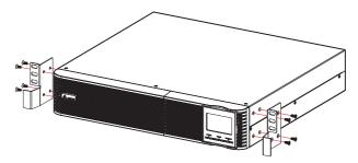
(Figure 3-1: Install the Ear bracket Kit)
