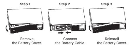
(Figure 4-1: Battery Cable Connection)
