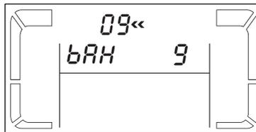
**Parameter 3:** Set the total battery Ah value of the UPS (unit: Ah).
