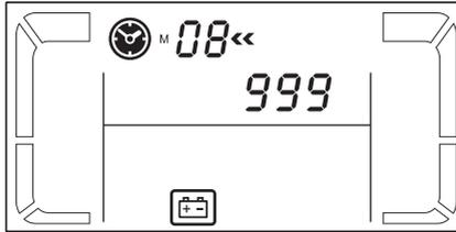
**Parameter 3:** Set the discharging time limitation in battery mode for general outlets.
