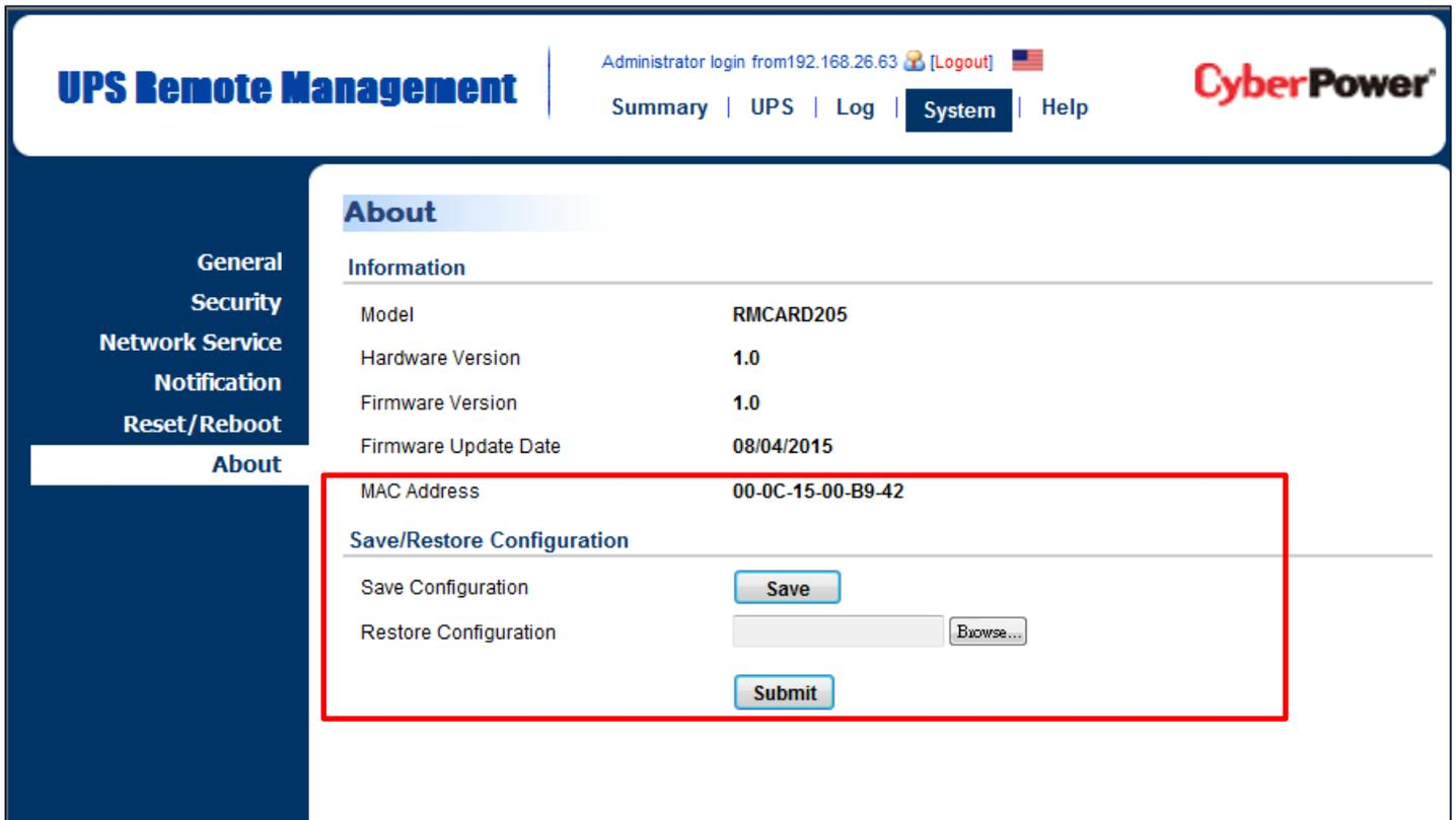
Figure 12. Save/Restore Configuration in the main window.
